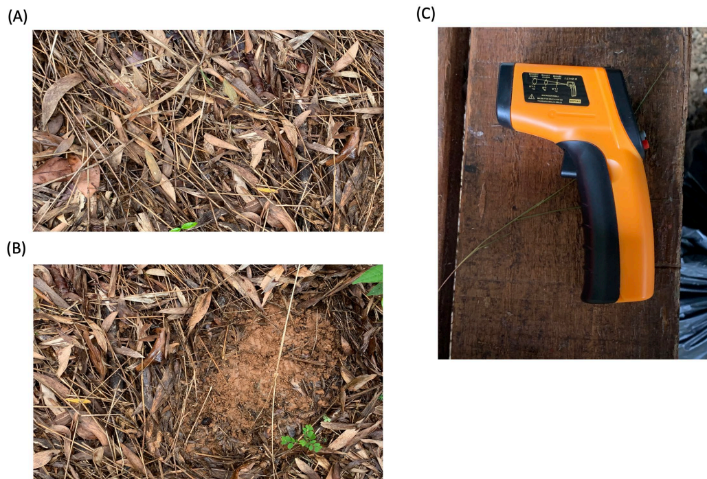
Figure 5: (A) Leaf litter-covered ground, (B) topsoil exposed by kicking the leaf litter away and (C) the infrared temperature gun used to measure the leaf litter and topsoil temperatures with a distance-to-spot ratio of 12:1.
