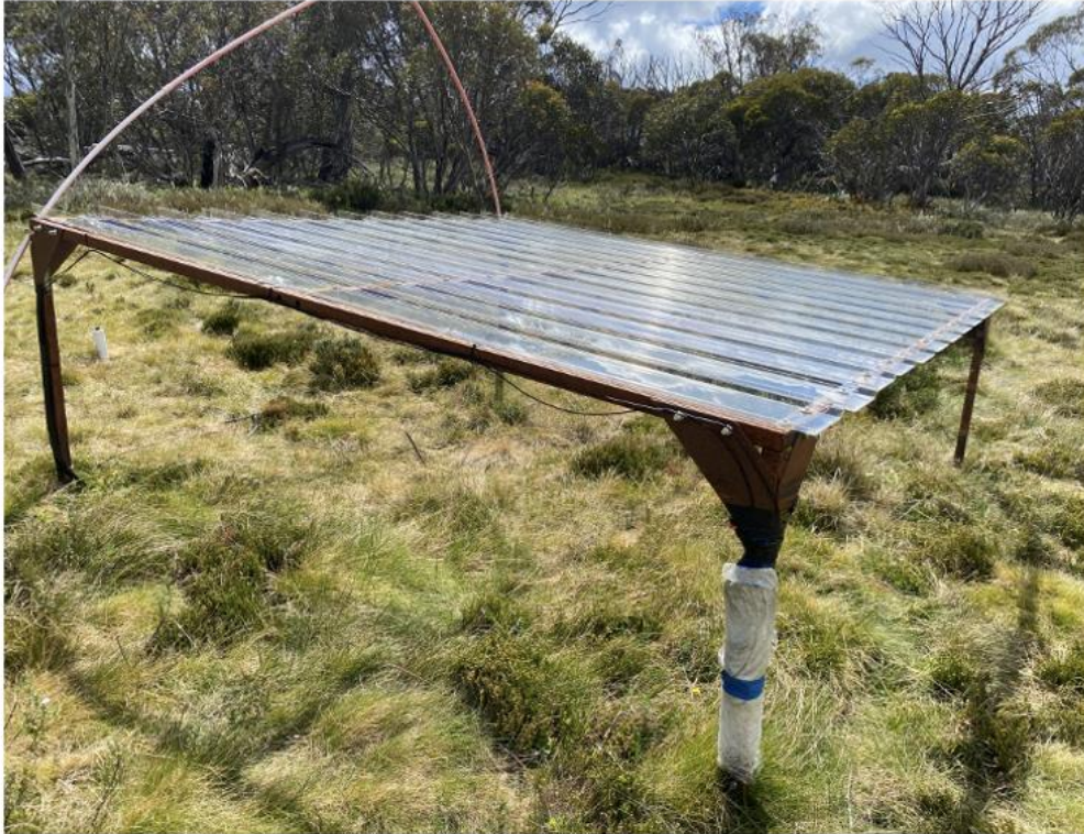
Figure 1. Drought shelters established by the Australian Mountain Research Facility, which divert 60% of incident rainfall.
